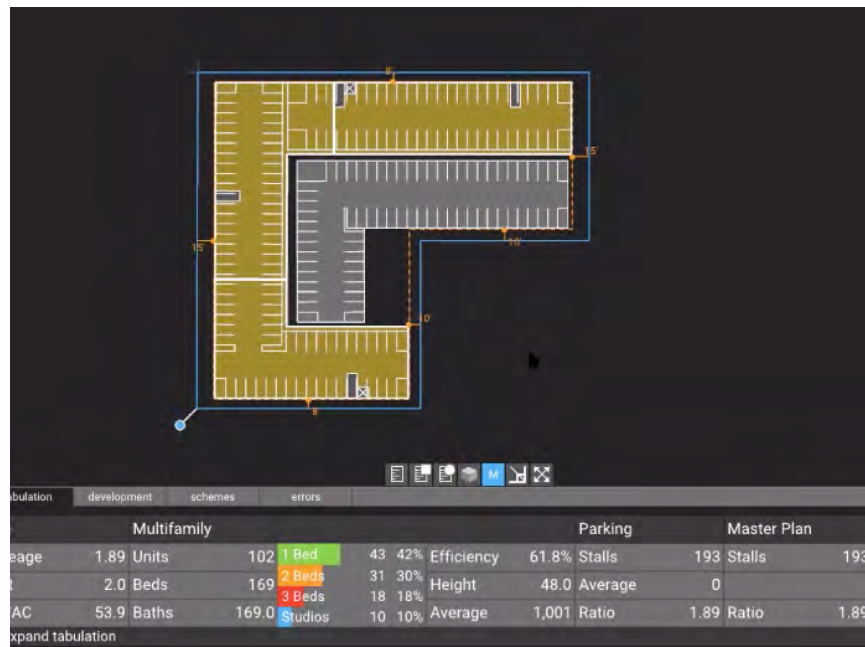
Figure 6.0 Utilizing TestFit's parking automation to determine if the ideal unit count was possible with the required parking ratio on the Beach Site.
